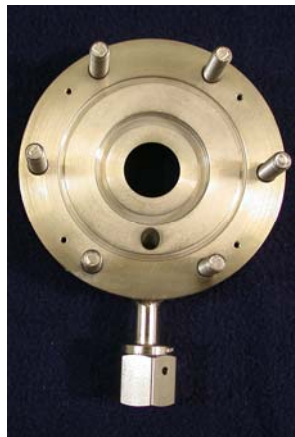
Figure 5 CRV half with bolts in place
